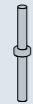
Connessione con collare tra gamba e colonna Connector with collar between leg and column
